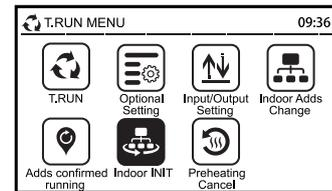
(3) Select the "Reset Indoor Adds" by pressing " ^ v " and press "☑".
