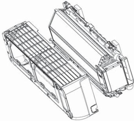
(3) There are four stoppers inside of the flat panel. Check to ensure that there is no gap between flat panel and unit body.
