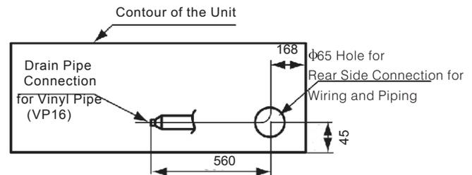
Fig. 6.1 07~17 Direction of Drain Piping
