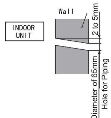
Fig. 4.2 Hole for Piping on the Wall
