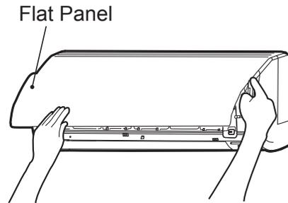
(2) Remove the air filter and six (6) screws. Slowly pull the lower side of the front panel and release the catch by paying attention to the air outlet part without touching the outlet grille.
