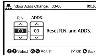
\* "R.N No.99" is used temporarily address only when all the cycle numbers and unit numbers are in use (occupied).
