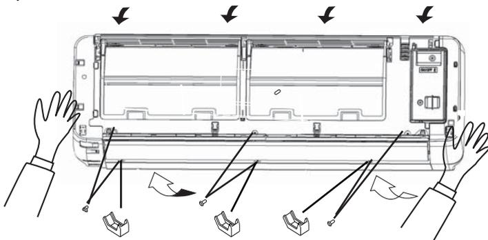
(2) Press flat panel down, make the two joints of the front panel tightly fasten.
