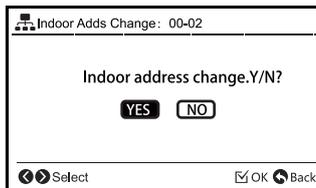
\*When the process successfully completes, "Adds Change Ended" will be displayed.
