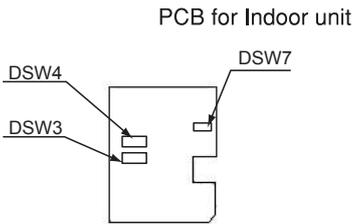
(B) The PCB in the indoor unit is equipped with 3 types of dip switches and rotary switch. Before testing unit, set these dip switches according to the following instructions.
