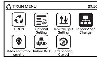
(2) Select "Indoor Adds Change" from the test run menu pressing " $\wedge \vee < >$ " and "☑".
