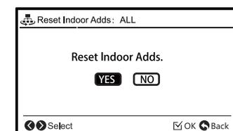
\*If the address initialization is successfully completed, connection check will be started automatically.
