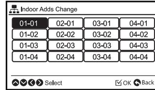
(3) Select the indoor unit by pressing " $\wedge \vee < >$ " and press "☑".
