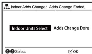
\*If "Indoor Adds Change" is successfully completed, connection check will be started automatically.
