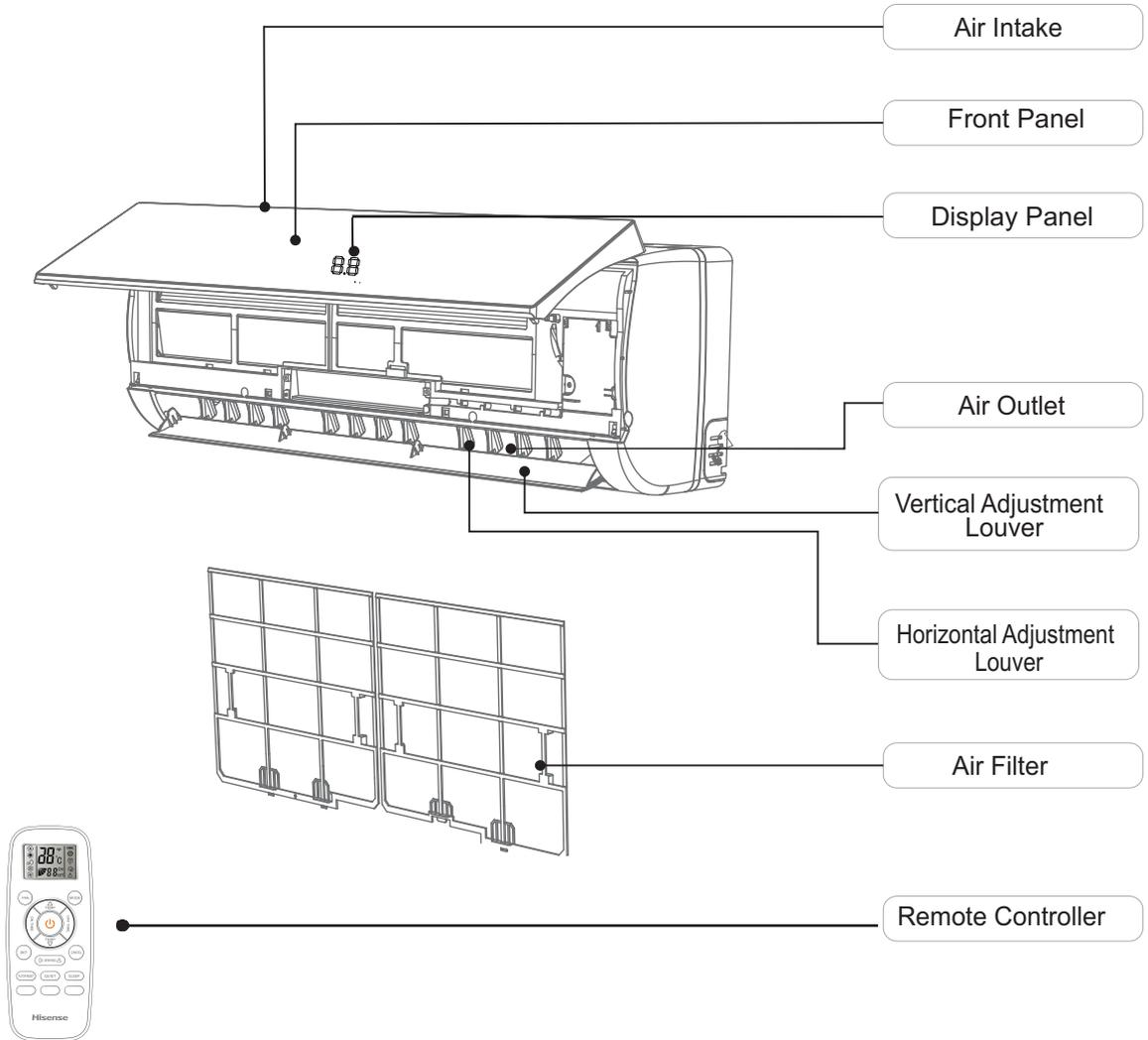
Fig.2.1 External Parts of System
