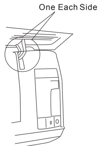
(4) Slightly lift the front panel upward in order to release the combined parts of upper side of the front pane
