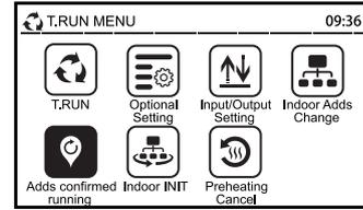
(2) Select "Adds confirmed running" from the test run menu pressing "< > ^ v < >" and "☑".
