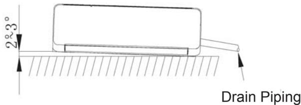
Fig 4.6 Slop angle of the Indoor Units
