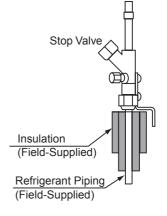
Fig. 8.2 Insulation on Pipes
