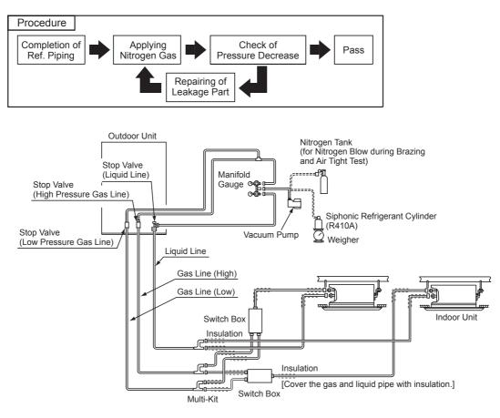
Fig. 8.1 Vacuum Pumping and Refrigerant Charge
