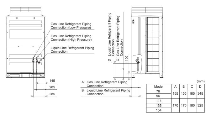
Fig. 6.1 Refrigerant Piping Connection
