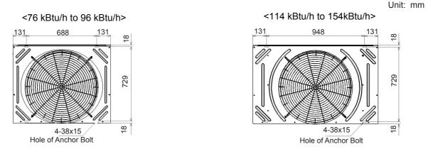
Fig. 5.1 Position of Anchor Bolts
