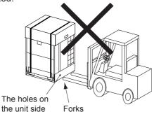
Do not apply excessive force to the square holes with forks or other materials. The bottom of the unit may be deformed.
