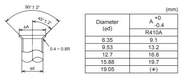
(\*) It is impossible to perform the flaring work with 1/2H material. In this case, use an accessory pipe (with a flare)
