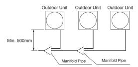
(6) Direction of Manifold Pipe Place the Manifold Pipe vertically towards the ground (within  $\pm 15^{\circ}$ ) as shown in the figure
