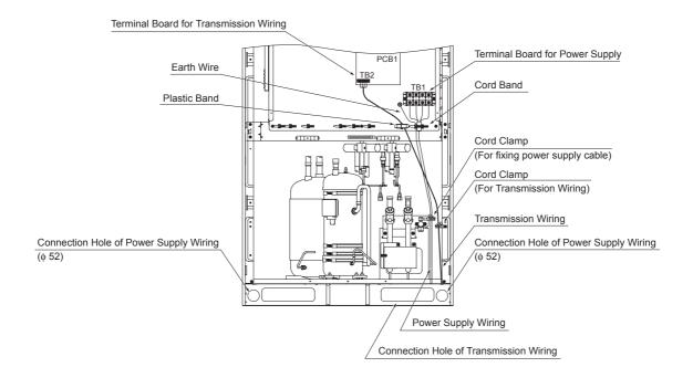
Fig. 7.1 Wiring Connection
