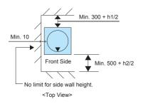
This indicates the direction of the unit (Front Side) when installing the units.
