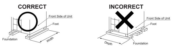
(3) Install the outdoor unit in the front-rear and right-left direction horizontally. (Use a level gauge.) Check to ensure that the gradient in four directions (front, rear, right and left) is within 10mm.
