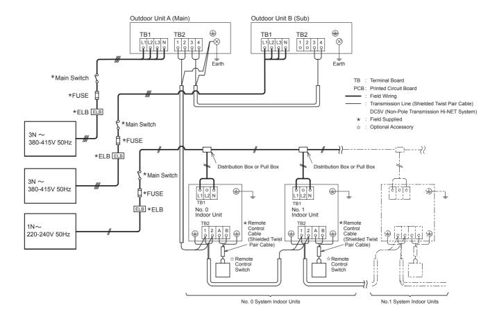
Fig. 7.2 Instruction for Electrical Wiring Connection
